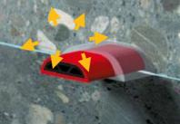
There are also SikaSwell® systems specifically designed to develop these swelling pressures with seawater and water with a high salt content.
